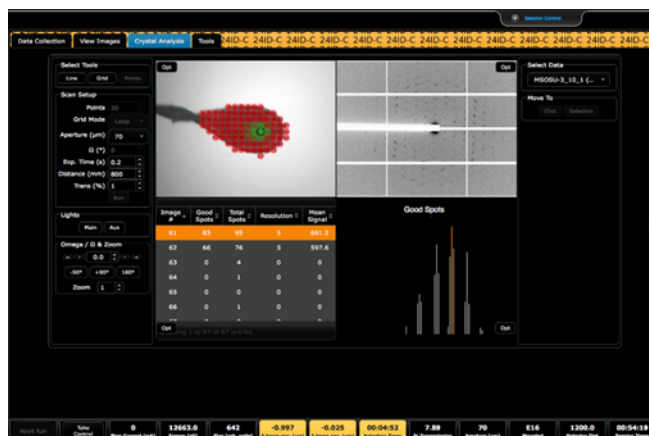
Fig. 3 New grid scanning technique in remote GUI. Highlighting an individual spot will show its location in the scan and in the histogram of peak heights. The central portion of the diffraction image for that spot will also be displayed.
