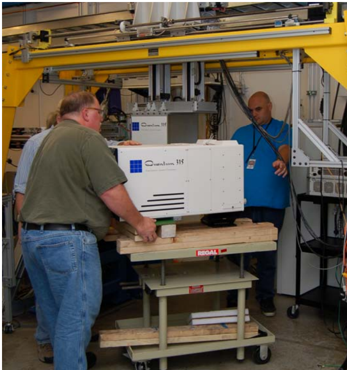
Figure 1. Q315 Detector being removed from the A-Frame in the 24-ID-E hutch in preparation for refurbishment.
