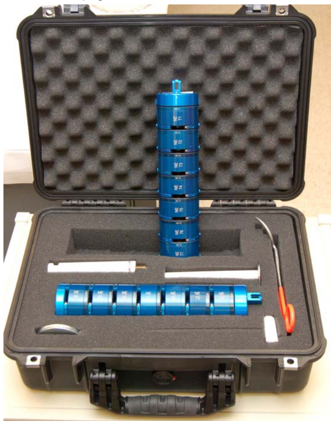
Figure 4. Shipping kit for loaner pucks. Kit includes cryopucks, shipping cane, shipping cane hook, bent cryopuck tongs, puck separator, puck wand and stand for stabilizing pucks.
